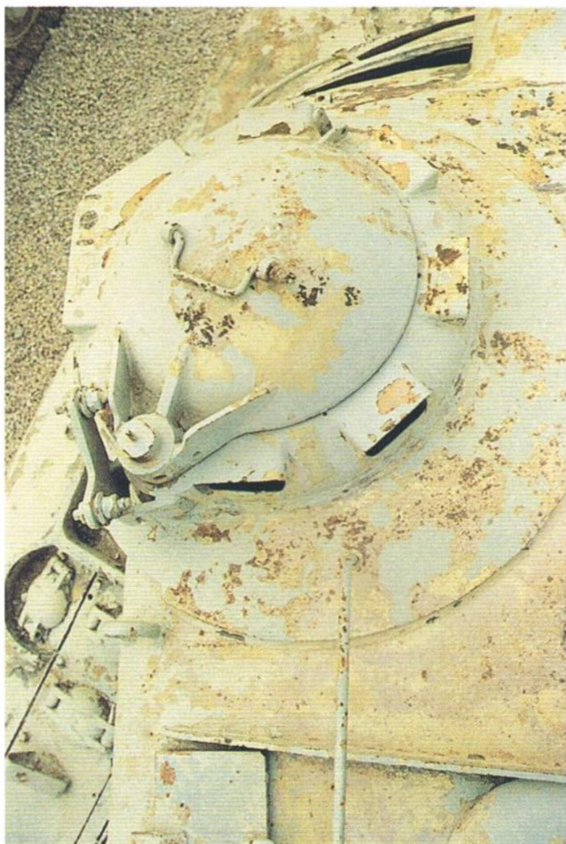
Fig. 5 The commander's hatch with its all-round vision blocks. Note the extra bracket next to the filler cap on the engine deck.
