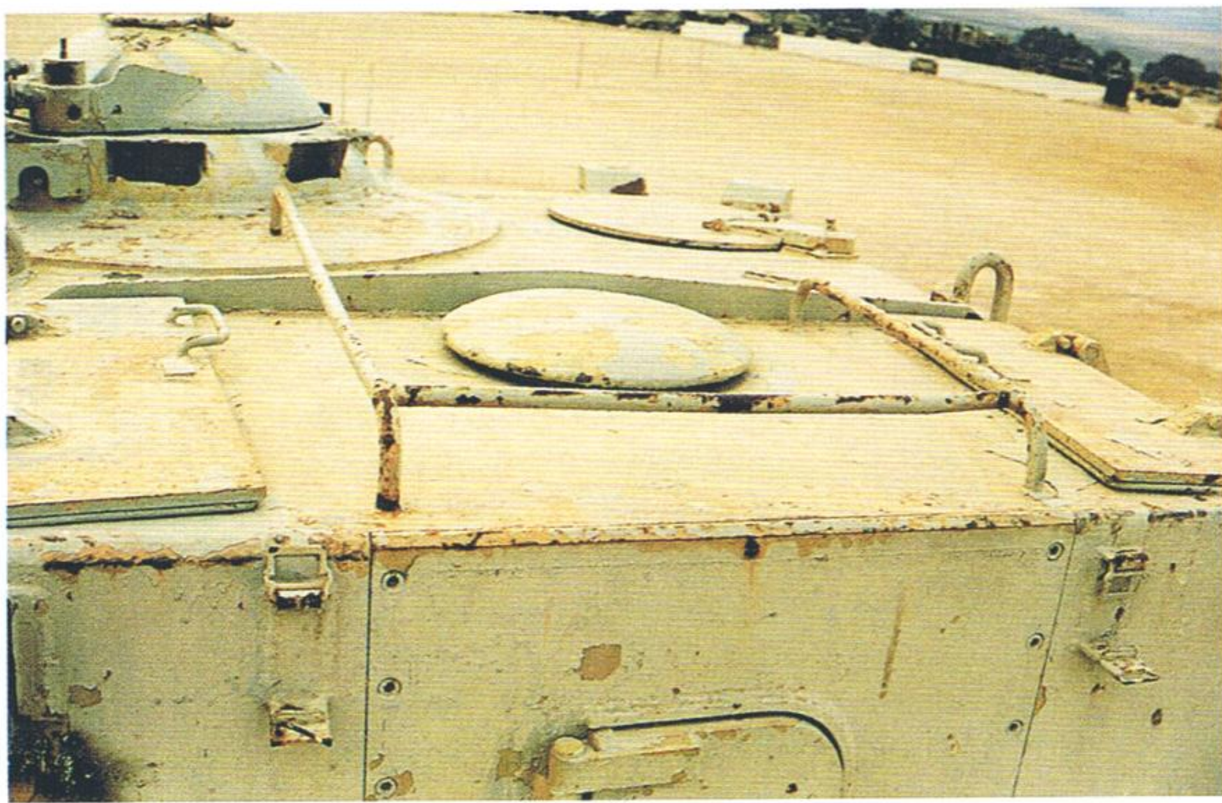
Fig.7 The upper rear of the turret with the two top hatches and the air/fume extractor in the middle. Note the shell discarding door at the rear.
