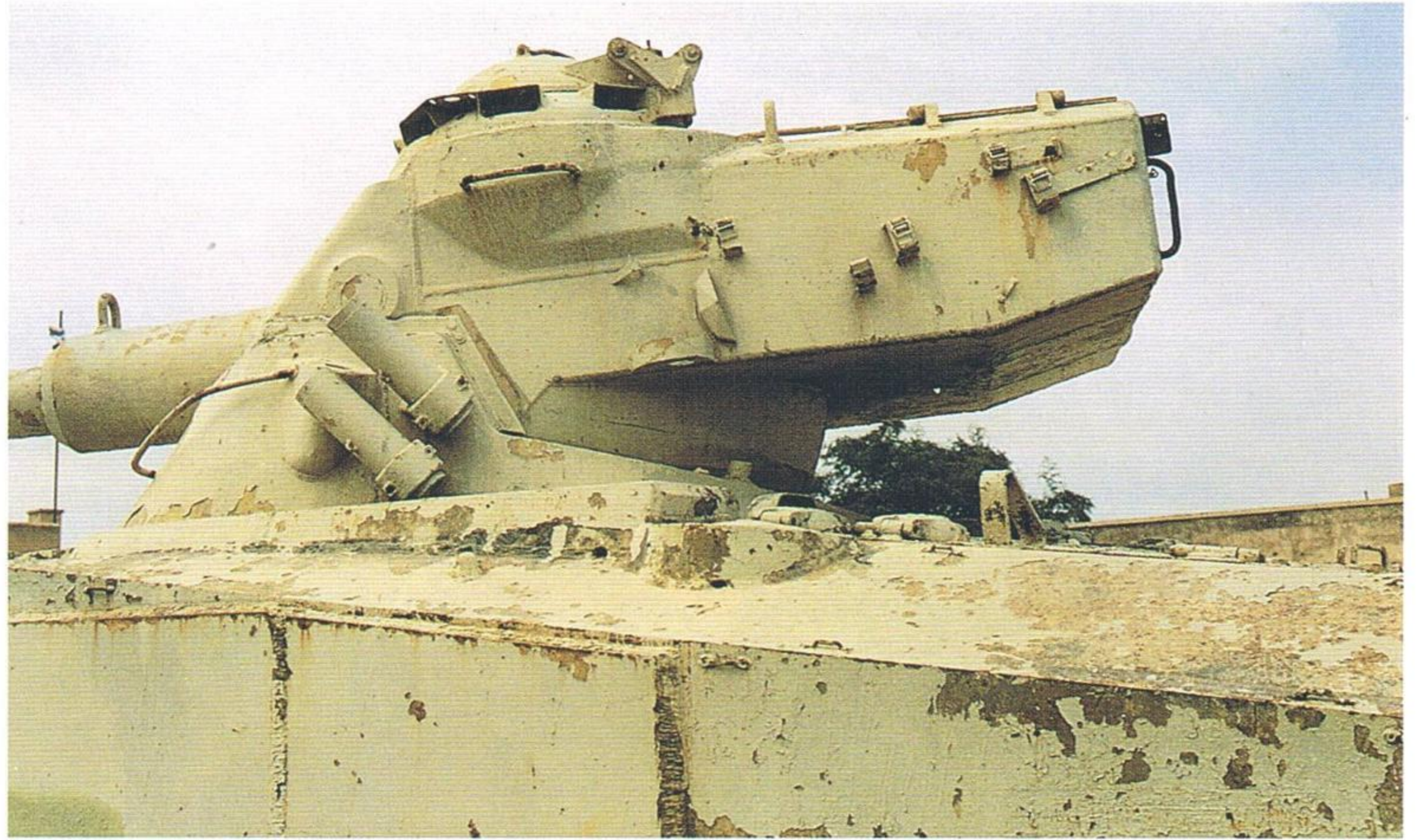
Fig. 11 A perfect look on the rear of the turret and turret bustle. The position and angle of the smoke grenade dischargers is evident. Note the commander's cupola extends some distance from the turret side wall. Brackets for an additional shovel and a non-identified tool are mounted on this side of the turret.
