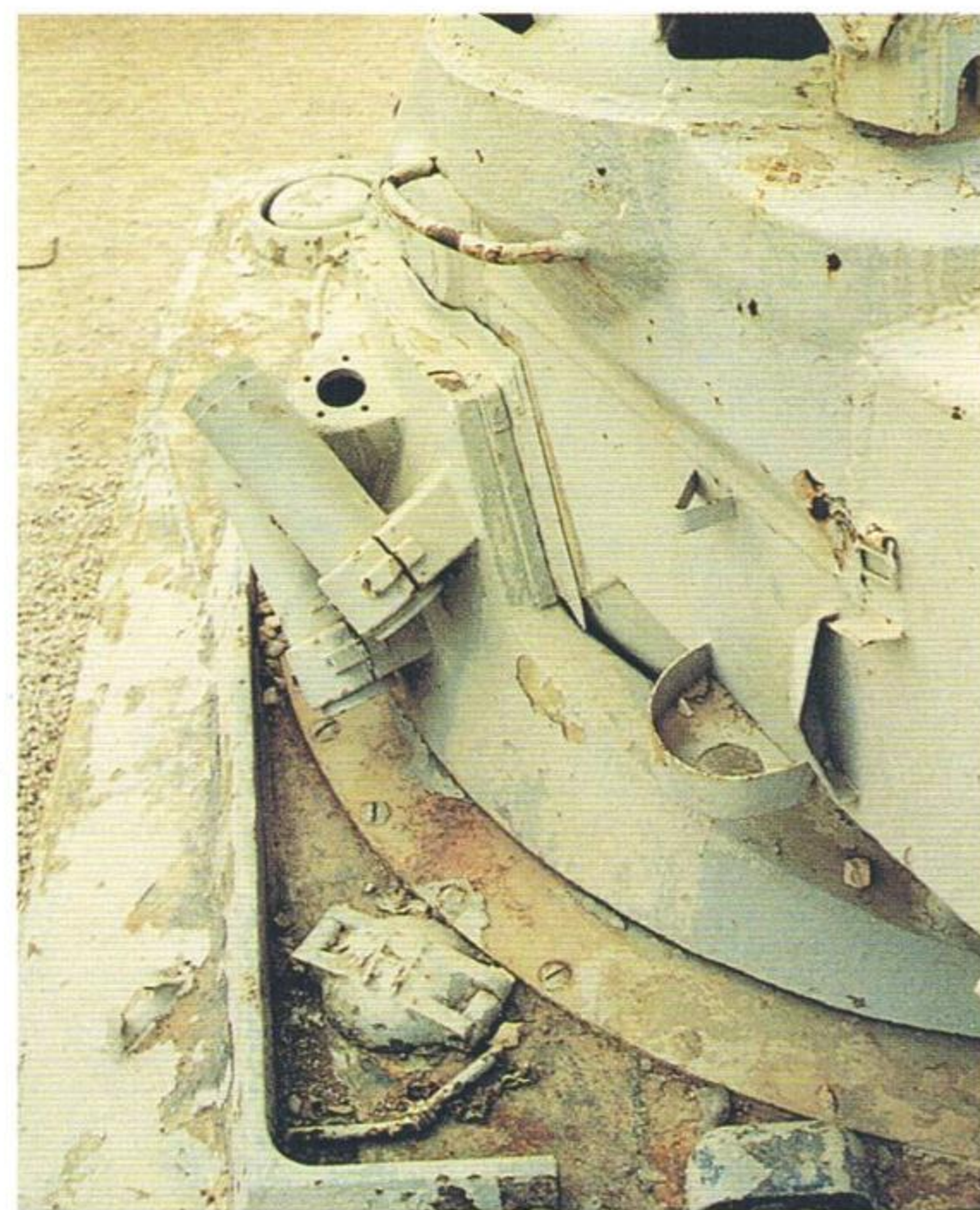
Fig. 6 A view on the left turret side of the real thing. Note the position and aiming direction of the smoke dischargers and the bracket on the lower edge.
