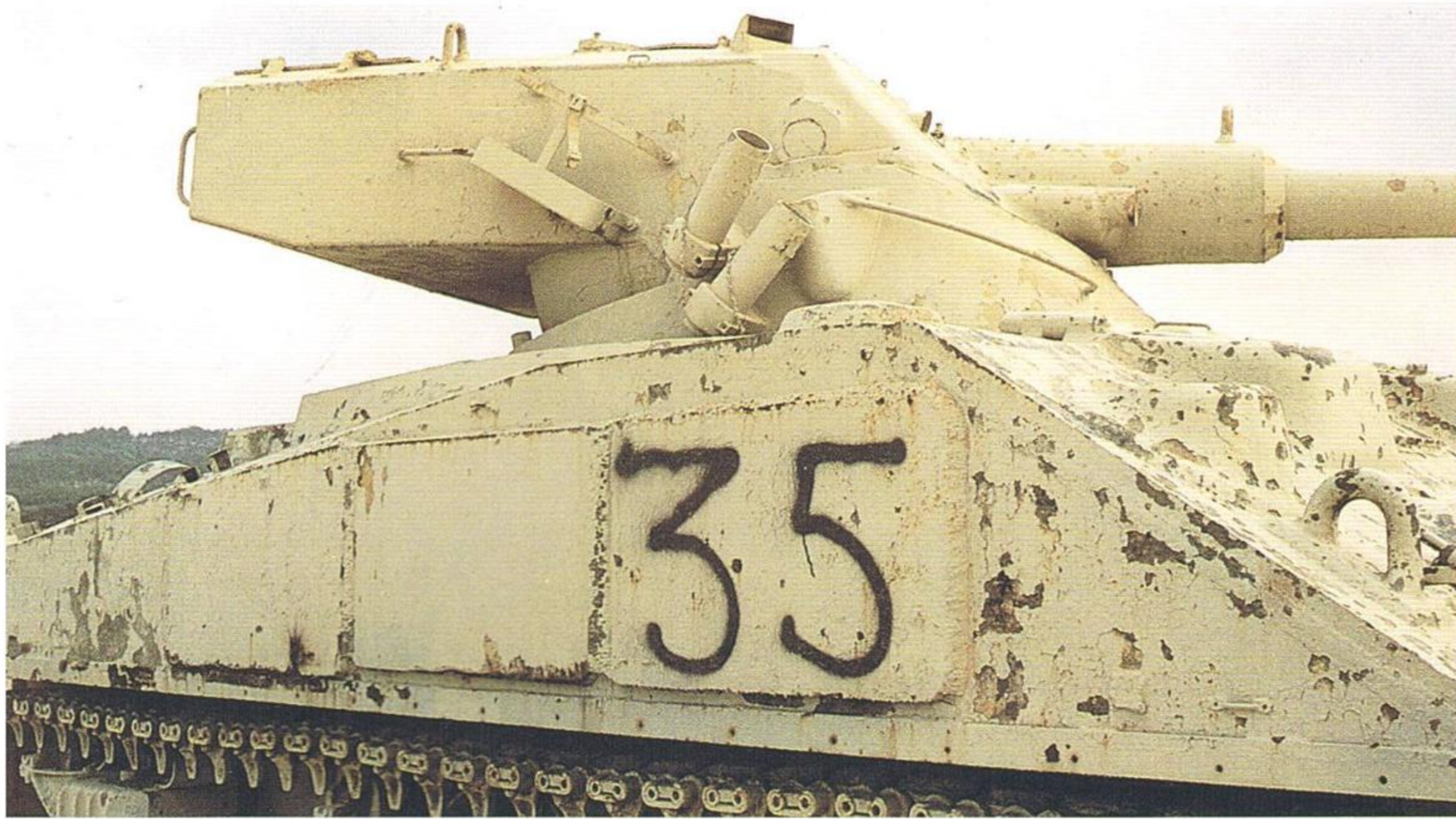
Fig.3 Hull and turret detail of the right side. Note the empty jerrycan holder on the turret. We preferred to have the jerrycan installed.
