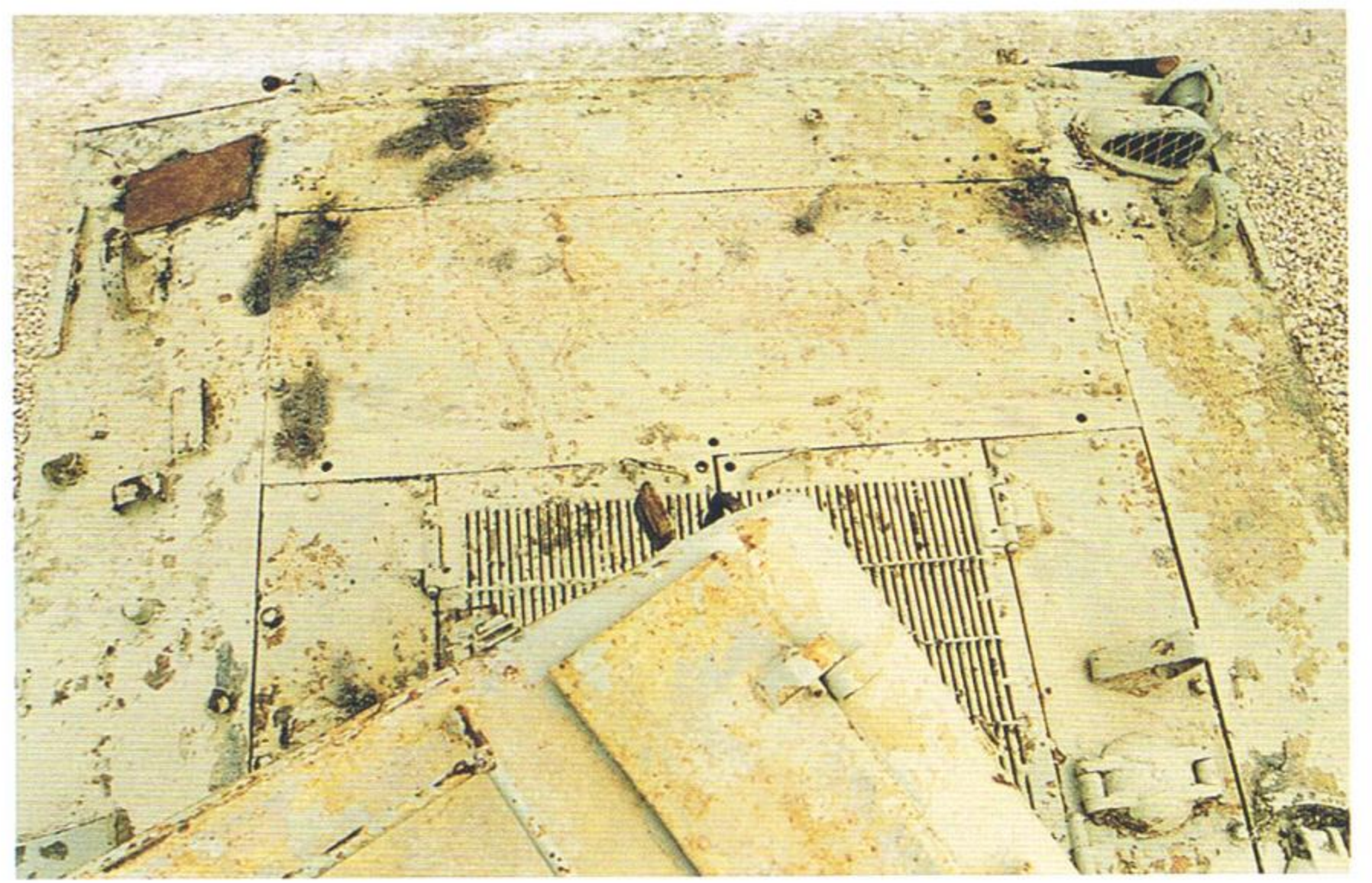
Fig.8 A view on the upper engine deck which is no different from a regular M4A2 deck except for the omission of the filler cap in the center aft of the access hatches.
